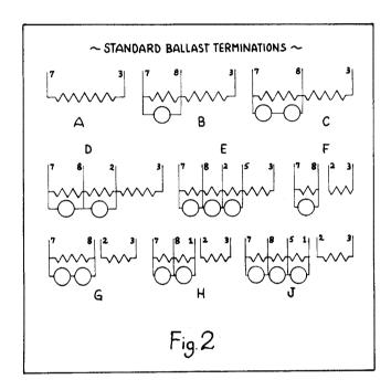
For example, Ballast type BK86A is an "A" type base wired unit. It is checked by referring to diagram "A" of Fig. 2, which reveals that lever 3 must be thrown to "F" position and then back to "NORMAL" position. Lever 7 must then be similarly actuated.
